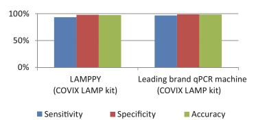
In a lab study done at Acibadem University using saliva samples taken from patients at the Acibadem Hospitals, LAMPPY was compared to a well-known conventional qPCR machine in performance and speed. The comparison study was carried out with a sample size of 262 using the COVIX LAMP-based kit on both instruments and then verified with the KrosQuanT SARS-COV-2 (2019 nCOV) Real Time PCR Diagnostic Kit on a leading brand conventional qPCR machine.
