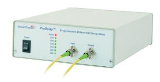
pin TTL digital I/O port to interface with any digital control signal, either from a control circuit board or a computer. Optional Labview PMD emulation software can also generate Maxwellian DGD distribution of any average value. In addition to PMD compensation and emulation, this patented device can also be used for precision TDM bit alignment.
