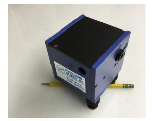
An optical beam traversing a uniformly rotating pair of parallel (//) mirrors encounters a time varying delay \*.
