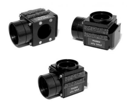
Exciter (x) = 20mm, Emitter (m) 20mm with a 2.5mm maximum thickness, Beamsplitter = 19x28mm. \*\*Recommend installation at Chroma to ensure proper gluing and alignment.
