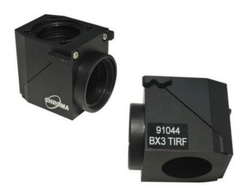
Laser TIRF for Olympus BX3/IX3 models, for 25mm filters
