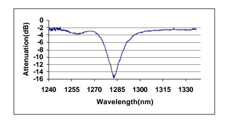
Long period grating couples light from a guide mode into forward propagating cladding modes where it is lost due to absorption and scattering. The coupling from the guided mode to cladding modes s wavelength dependent so we can obtain a spectrally selective loss.
