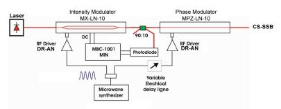
Efficient Single Side Band modulation and Carrier Suppression can be achieved by using a combination of Intensity and Phase modulators properly driven with DR-AN analog RF amplifiers.
