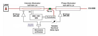
Efficient Single Side Band modulation and Carrier Suppression can be achieved by using a combination of Intensity and Phase modulators properly driven with DR-AN analog RF amplifiers.
