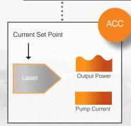
ACC (Automatic Current Control) mode is standard for all devices. The laser is controlled from diodes current set point.
