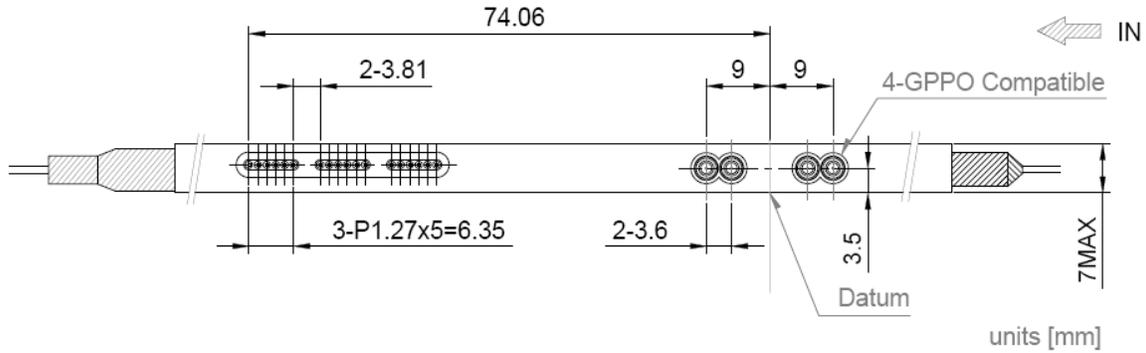
Figure 4. Mechanical specification of DC and GPPO RF interfaces
