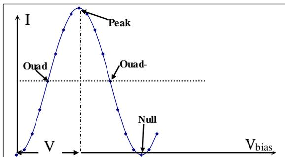
Figure 1. Modulator working function
