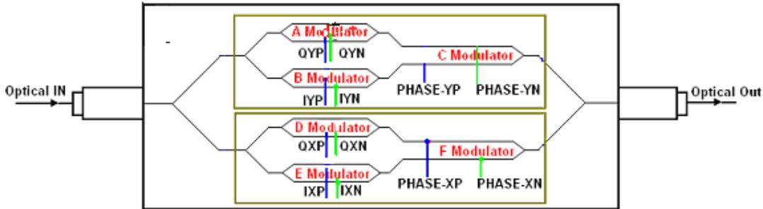
Figure-3 DP QPSK modulator numbering for 0157F MBC
