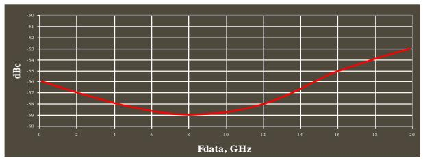
Fig. 5. 3-rd Harmonic at 4GHz Input Clock (C) and 125mV Differential Data (D) Amplitude
