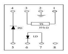
330mW Kink-Free, FBG Stabilized, 980nm Uncooled Pump Laser Module
