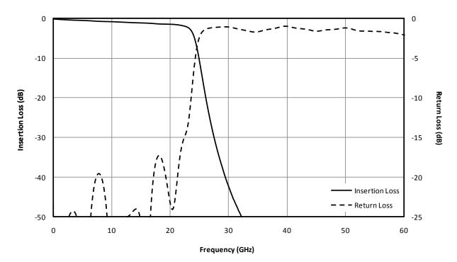
Fig. 1. Magnitude response for a typical FLP-2360.
