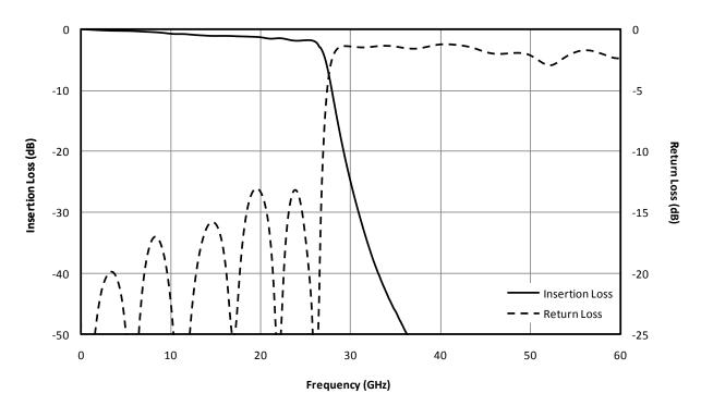
Fig. 1. Magnitude response for a typical FLP-2650.
