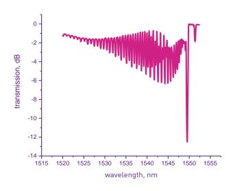
outside the fiber cladding. TFBGs are useful in sensing applications. Possible value of tilt angle is  $1^{\circ}$  -  $45^{\circ}$ . The TFBG transmission spectrum of 10mm length with tilt angle of  $3^{\circ}$  is presented in the graph.
