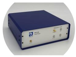
The unique design of the OEwaves HI-Q® VCO is based on photonic generation of spectrally pure signals at millimeter wave frequencies with *phase noise that is independent of output frequency*. This is accomplished with patented technology of semiconductor lasers injection locked to ultrahigh quality factor (Q) crystalline optical whispering gallery mode resonators.
