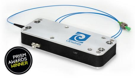
The HI-Q<sup>®</sup> laser houses a proprietary driver/controller and the OEwaves laser source which is based on a high quality factor (Q) Whispering Gallery Mode (WGM) optical micro-resonator. The laser is available at a variety of wavelengths (370 - 4500 nm).
