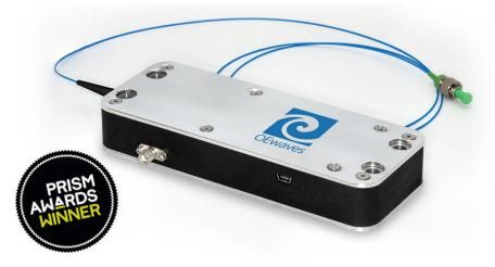
This HI-Q<sup>®</sup> laser houses a proprietary driver/controller and the OEwaves laser source which is based on a high quality factor (Q) Whispering Gallery Mode (WGM) micro-resonator. The laser is available at a variety of wavelengths in the 780nm region.
