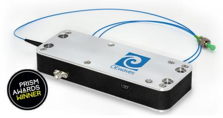
This HI-Q® Laser houses a proprietary driver/controller and the OEwaves laser source which is based on a high quality factor (Q) Whispering Gallery Mode (WGM) micro-resonator. The laser is available at 1064 nm. Other nearby wavelengths available by custom order.
