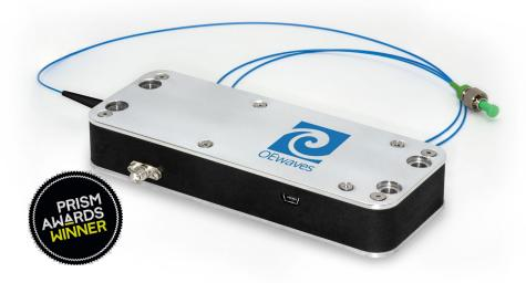
This HI-Q® Laser houses a proprietary driver/controller and the OEwaves laser source which is based on a high quality factor (Q) Whispering Gallery Mode (WGM) micro-resonator. The laser is available at a variety of wavelengths within 1900 – 2100 nm.
