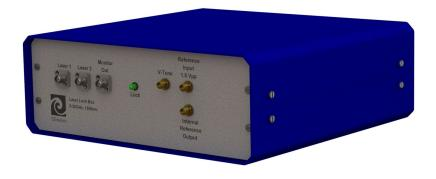
HI-Q® Laser Phase Lock System is capable of automatically and rapidly phase locking two lasers together with a simple setup. The Locker outputs the locking voltage for feedback to the source laser's frequency tuning port such as the piezo tuning port of an OEwaves OE4030 Hi-Q® sub-Hertz laser.
