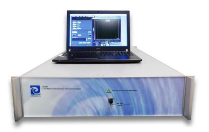
HI-Q<sup>®</sup> RIN Analyzer is capable of automatically and rapidly measuring relative intensity noise spectrum without complex setup.
