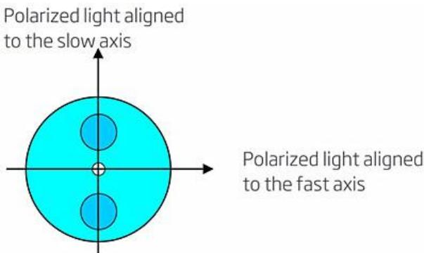
Note: The PM fiber and the connector key are aligned to the slow axis, fast axis is blocked.
