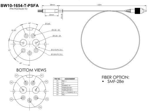
CAUTION: Device is sensitive to electrostatic discharge.
