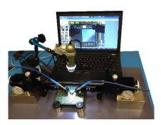
Horizontal probing of RF module and circuit board
