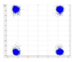
Figure 4. QPSK Constellation(with controller)
