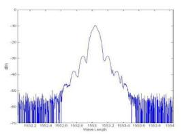
Figure 6. QPSK Spectrum
