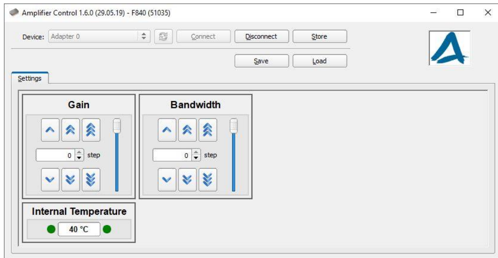
GUI of the SHF Amplifier Control software V1.6
